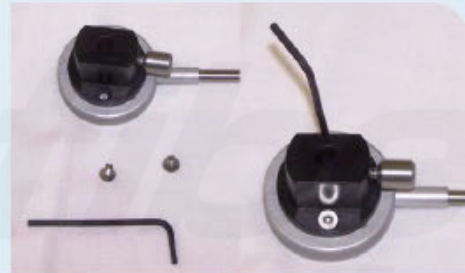
Figure 5. Attach Lightguide Adapter to Lightguide (Step 4)
