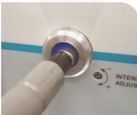
Figure 6. Insert Lightguide into Lightguide Mount
