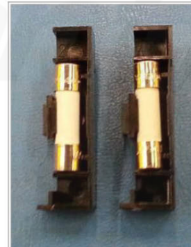
Figure 52. Fuses Removed from Holder
