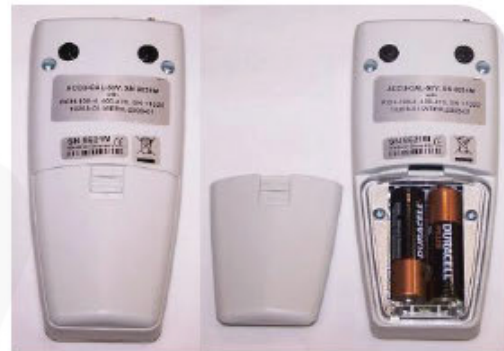
Figure 7. Battery Compartment (Closed & Open)
