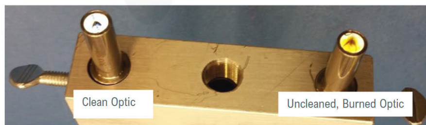
Figure 4. Damaged, Burned Lens
