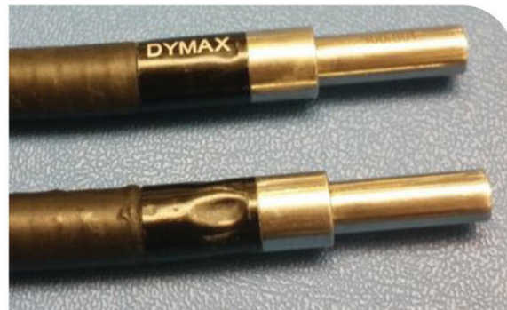
Figure 8. Damaged Lightguide Caused by Over Tightening
