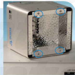
Figure 2. Remove Screws from Reflector
