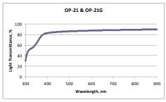
\*Measured at 0.03 mm [0.001in] per DSTM-501
