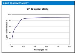
Measured at 0.03 mm [0.001" in] per DSTM-501<sup>‡</sup>
