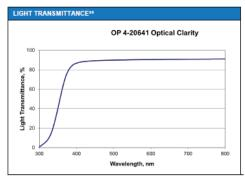
Measured at 0.03 mm [0.001" in] per DSTM-501\*
