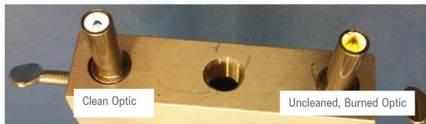
Figure 4. Damaged, Burned Lens
