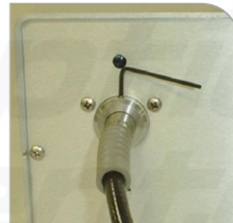
Figure 2. Tighten Set Screw with Hex Wrench
