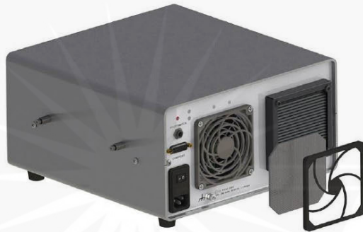
Figure 48. Intake Fan with Fan Filter Remove
