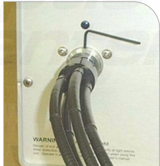
Figure 2. Tighten Set Screw with Hex Wrench
