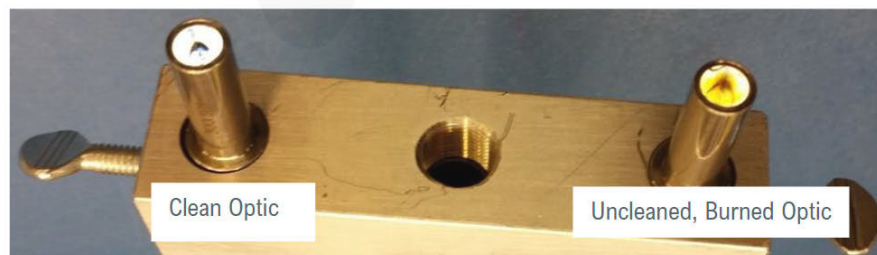
Figure 4. Damaged, Burned Lens
