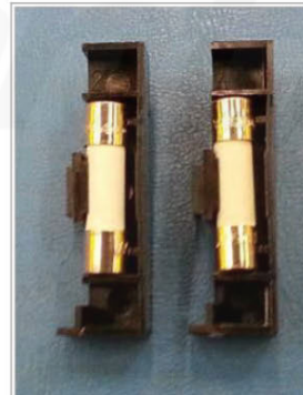
Figure 52. Fuses Removed from Holder
