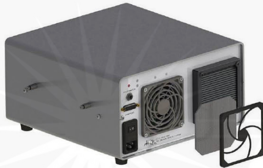
Figure 48. Intake Fan with Fan Filter Remove
