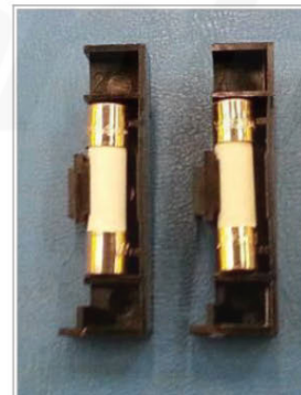
Figure 52. Fuses Removed from Holder
