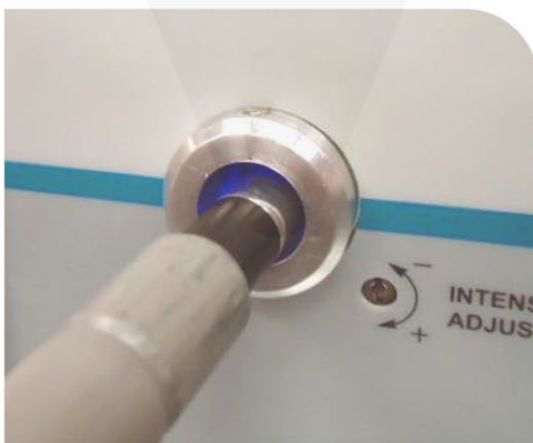
Figure 6. Insert Lightguide into Lightguide Mount
