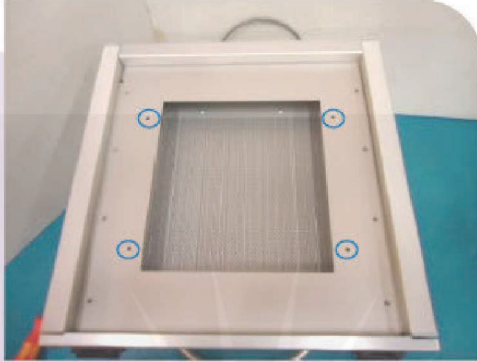
Figure 6. Remove Screws from Light Shield Top Cover
