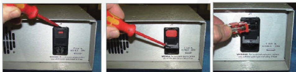
Figure 10. Replacing Fuses in the Power Supply
