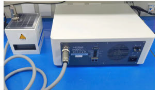
Figure 7. Interconnect Cable Installed
