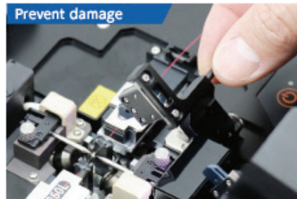
Prevent damage Releasing the fiber clamp links allow the fiber clamps to be placed without closing the canopy.
