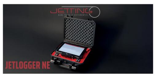
JetLogger NE is a professional documentation system for the installer who need an efficient and professional electronic documentation of the cable blowing process. Jetlogger is developed together with installers, network owners and approved by German Telecom - ZTV TKNetz 40. Jetlogger can be delivered to following models: V0- V0 HD- V2 and V3.
