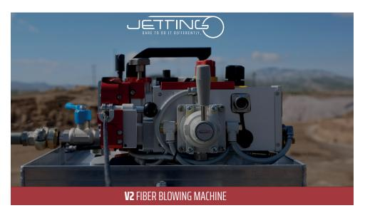
Robust and compact pneumatic operated fiber blowing machine with the unique Joystick controller securing optimal control of the installation. This machine can be configurated from 2,4 to 16 mm cable and 7 to 50 mm duct. Anodized aluminum construction makes this machine both lightweight and easy to maintain .
