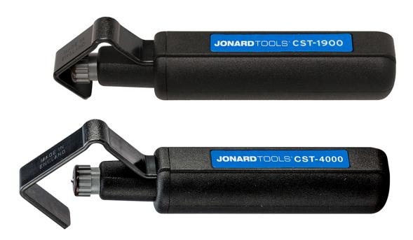
The **PATENTED** CST-1900 and CST-4000 Round Cable Strip & Ring Tools are designed for fast and precise removal of cable jackets from round cables. The CST-1900 removes cable jackets 3/16" to 1 1/8" (4.5 mm to 29 mm) in diameter and the CST-4000 removes cable jackets 3/4" to 1 5/8" (19 mm to 40 mm) in diameter. These round cable strippers feature the following:
