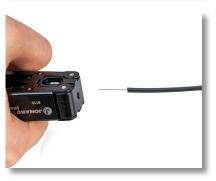
Specifically designed to strip FTTH drop cables sized 1.6 mm (**FDS-216**) and 3.1 mm (**FDS-312**) by 2.1 mm. These drop cable strippers strip the outer jacket of drop cables and cuts the strength members to expose the fiber inside. These drop cable strippers feature the following:
