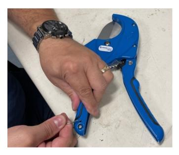
2. Unscrew the 2 screws of the rigid handle and remove the grip
