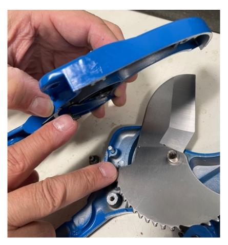
8. Fit the faceplate back onto the unit it snaps into place and replace the assembly.
