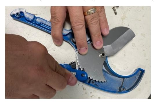
7. Position the torsion spring so that it is contacting the flat part of the back of the blade
