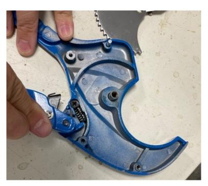
6. While holding the moveable handle in place, put the new blade into the housing
