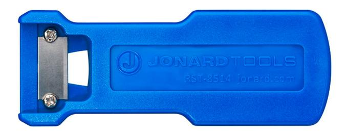
Designed to shave a longitudinal access window in round FTTH riser cables and microducts, this riser slitting tool is perfect for making access windows on cables 8 to 14 mm (0.33" to 0.55") in diameter without damaging the fiber inside. This tool features the following:
