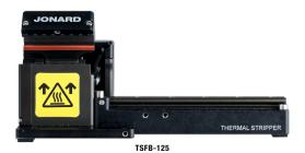
The Jonard Thermal Strippers are compact, easy-to-use fiber stripping units designed to thermo-mechanically remove coatings from optical fibers. The heater is adjustable up to 200°C; far hotter than any competing product. This feature facilitates stripping extremely difficult and baked-on coatings and in some cases can even remove fluoroacrylate undercoatings.
