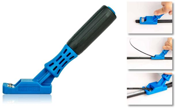
Designed to shave a longitudinal access window in round FTTH riser cables and microducts for mid-span access. This riser slitting tool is perfect for making access windows on cables 8 to 14 mm (0.33" to 0.55") in diameter without damaging the fiber inside. This tool features the following:
