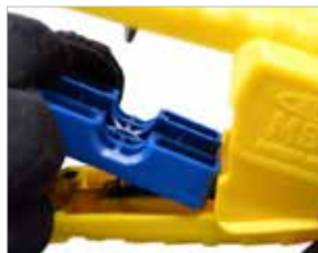
Magnetic trays accurately determine the appropriate blade depth & cable diameter to prevent damage.
