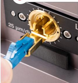
Hold the epoxied ferrule or connector at its base and carefully insert it into the Adapter Hole as far as it will go.
