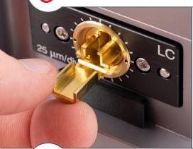
Some Single Fiber adapters require specific orientation in order to cut properly. For all necessary adapter orientations, see User Information: Connector and Ferrule Adapters.
