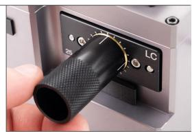
Adjusting Ring clockwise to cut closer to the ferrule face, counterclockwise to cut further away. Each calibration mark on the Adjusting Ring represents a 25  $\mu$ m distance. The cut distance can be set between calibration marks for an even finer adjustment.
