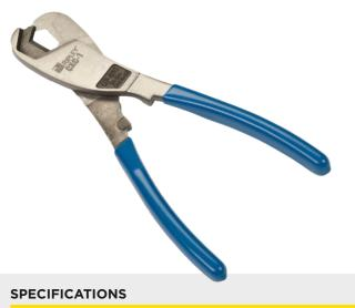
Cuts efficiently through aluminum trunk & distribution coaxial cables without cable distortion
