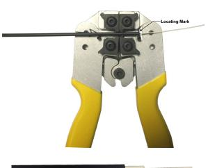
Squeeze the handles fully to cycle the tool and the specified length of jacket material will be removed exposing the GPR rods.
