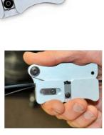
Cable sits flat in the slitter channel with the toner wire against the blade, then close tool and slide to quickly separate.
