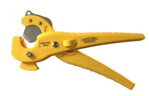
The Miller® MC02-7000 Duct Cutter is designed to make clean, square, and burrfree ring cuts in plastic fiber ducts up to 25 mm diameter. This duct cutter is ideal for cutting or scoring PVC, CPVC, HDPE, and other plastic tubing while protecting the inside fibers.
