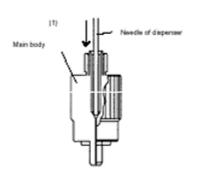
Step 1 Insert the needle of the dispenser into the main body of the plug from the tail until the dispenser stops.
