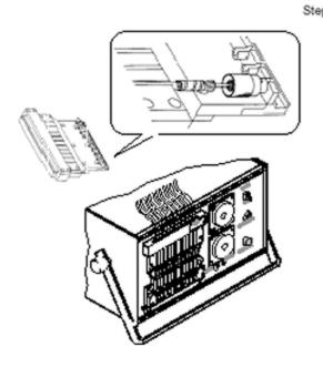
Step 1 Install the curing machine upside down as shown in the figure. Set the plugs on the cassette magazine and mount the cassette magazine on the OFK-1 curing machine. Adjust the temperature scale to 120 on the curing machine to harden the Epo-Tek 353ND. A maximum of 10 plugs can be cured at a time in the OFK-1 (For more details, see the curing machine manual).
