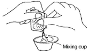
Step 1 Mix the main and curing agents of the adhesive Epo-Tek 353ND according to the instructions printed on the package of Epo-Tek.
