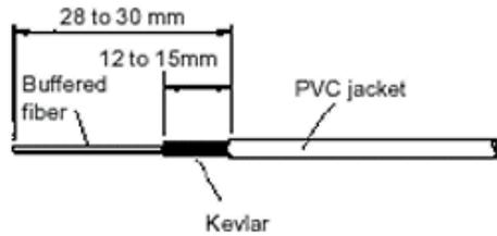
**Step 1** Using the wire stripper, Kevlar scissors and a scale, cut off the PVC jacket and the Kevlars to the length shown.
