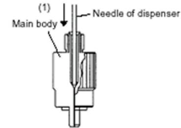
Step 1 Insert the needle of the dispenser into the main body of the plug from the tail until the dispenser stops.
