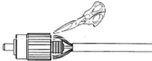
Step 1 Remove the spiral tube with care. Trim the Kevlars at the position shown in the figure with the Kevlar scissors.
