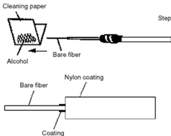
**Step 4** Wipe off the residual coating with a piece of cleaning paper moistened with ethyl alcohol.
