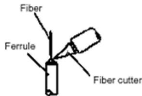
**Step 2** After completion of the hardening, cut the fiber projecting from the face of the ferrule by making a notch by a slight touch of the fiber cutter and then lightly bending the fiber down to remove it.
