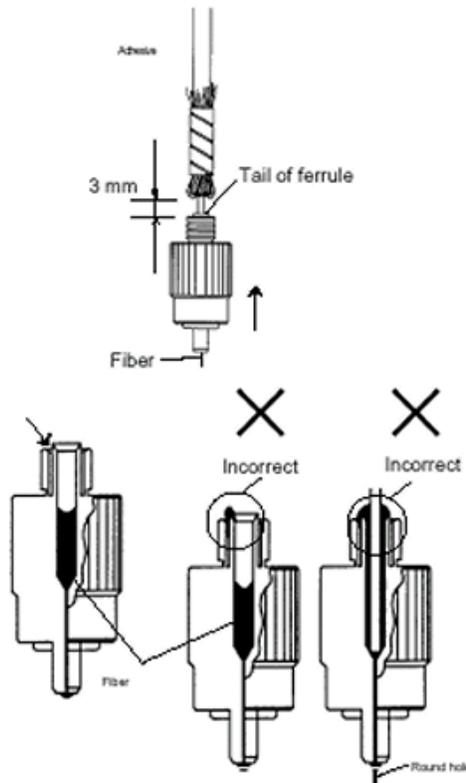
Step 5 Slide the plug onto the fiber slowly. Wipe off the excessive adhesive coming out of the tail of the ferrule.
