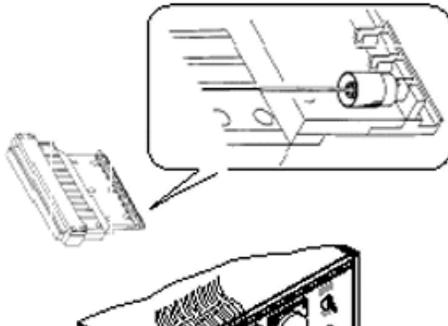
**Step 1** Install the curing machine upside down as shown in the figure. Set the plugs on the cassette magazine and mount the cassette magazine on the OFK-1 curing machine. Adjust the temperature scale to 120 on the curing machine to harden the Epo-Tek 353ND. A maximum of 10 plugs can be cured at a time in the OFK-1 (For more details, see the curing machine manual).
