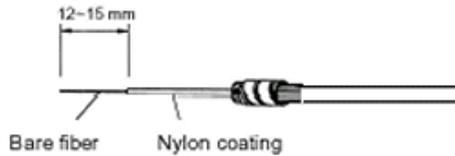
**Step 3** Using the fiber stripper and a scale, remove 12 to 15 mm of the nylon coating from the end of the cord as shown.
