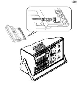
Step 1 Install the curing machine upside down as shown in the figure. Set the plugs on the cassette magazine and mount the cassette magazine on the OFK-1 curing machine. Adjust the temperature scale to 120 on the curing machine to harden the EpoTek 353ND. A maximum of 10 plugs can be cured at a time in the OFK-1 (For more details, see the curing machine manual).
