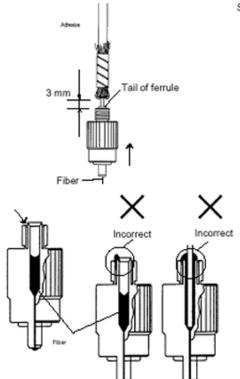
Step 5 Slide the plug onto the fiber slowly.
