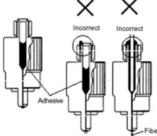
Take care so that adhesive will not pour into the part of the plug indicated by the arrow in the figure. Never
