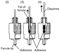
Step 2 Turn on the dispenser and inject adhesive until it comes out of the tip of the ferrule.
