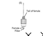
Step 5 Slide the plug onto the fiber slowly. Wipe off the excessive adhesive coming out of the tail of the ferrule.
