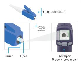
Debris on an end face is typically  $2-20 \mu m$  and can only be seen with a fiber optic probe microscope.
