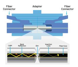
Inspecting BOTH sides of the fiber connection is the only way to ensure that it will be free of contamination and defects, and prevents cross-contamination. VIAVI fiber optic probe microscopes allow inspection of both male and female optical connectors.
