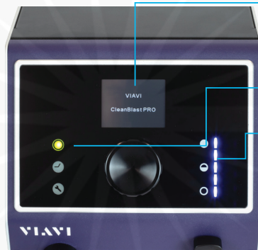
Figure 3: Front panel indicators and controls
