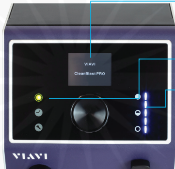
Figure 3: Front panel indicators and controls
