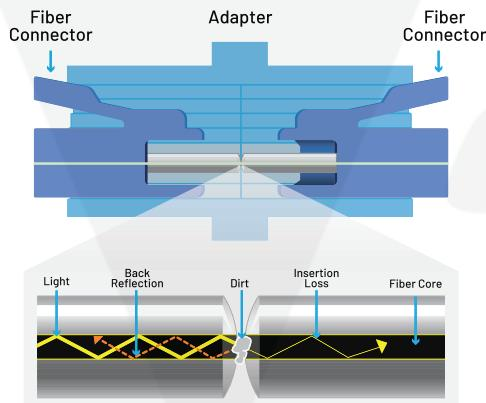
Inspecting BOTH sides of the fiber connection is the only way to ensure that it will be free of contamination and defects, and prevents cross-contamination. VIAVI fiber optic probe microscopes allow inspection of both male and female optical connectors.
