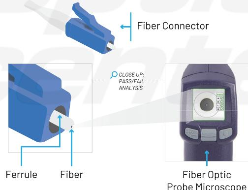
Debris on an end face is typically 2 - 20  $\mu\text{m}$  and can only be seen with a fiber optic probe microscope.
