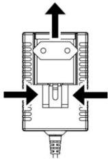
Fig. 3: AC line plug adapter
